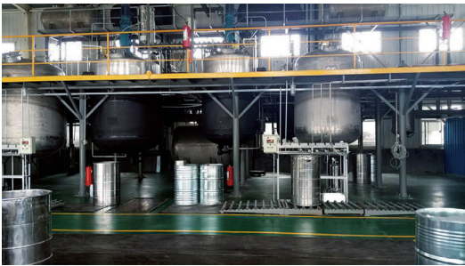
5 千吨/年新型离子液体电解液生产线 Production line of lithium battery electrolytes with ILs as additives (capacity: 5,000 tons/a)
