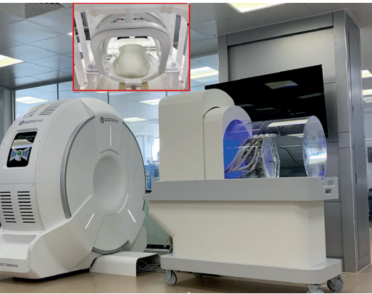
世界首台磁共振引导超声脑刺激仪器 The world's first magnetic resonance guided ultrasonic brain stimulation system
